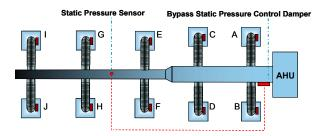
Balancing the  $T_3SQ$  VAV system is simple. First, drive open all diffusers. For the thermal  $T_3SQ$  this is done by disconnection the actuator arms from the control disc. For the analog  $T_3SQ$ , press and hold the down arrow to put the diffuser in override mode, signified by a LI on the thermostat display, then press the down arrow once to drive the control disc open.
