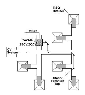
In discharge pressure control applications, the static pressure tap should be placed downstream of the terminal about 1/2 to 2/3 the way down the duct run.
