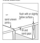
Clean subfloor and leave free of dust, dirt and debris. Ensure that subfloor is completely dry (no more than 12% moisture in subfloor prior to installation). Verify that fasteners are flush with, or slightly below, subfloor surface.
