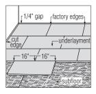
Prior to installation of final floor covering, avoid heavy traffic and moving heavy items across panels. If necessary, items such as refrigerators or other appliances with wheels (or on wheeled dollies) may be rolled over underlayment surface; using strips of hard wood or scrap underlayment to bear the wheel traffic is recommended. Allow a minimum of 24 hours after floor covering installation before placing heavy appliances or furniture on floor.
