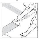
Prefill all joints with tile-setting mortar or adhesive, then immediately embed Durock interior tape over joints. Strike joints flush.
