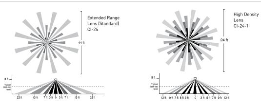
Coverage shown is maximum and represents coverage for half-step walking motion. Under ideal conditions, with no barriers or obstacles, coverage for half-step walking motion can reach up to 1200 ft2 using the Extended Range lens and up to 500 ft2 using the High Density lens. For typical desktop level of activity, coverage can reach up to 300 ft<sup>2</sup> using the High Density lens.
