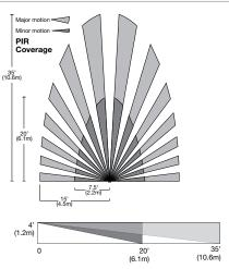
\* For best performance, WattStopper recommends using this sensor in spaces no larger than 15' x 12'.
