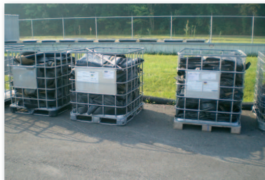
The removed EPDM roofing material is packaged for processing, then blended into R2R silicone coatings.
