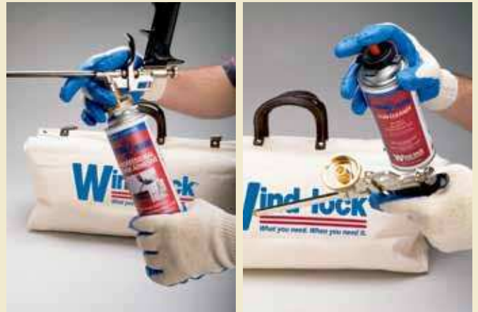
2. The can should point up and away from your face.
