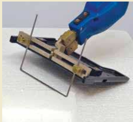
6. The Q-SLED6's adjustable blade depth is used for plunge or scooping cuts. The Q-EBX4 (Electrical Box Cutter) is shown.
