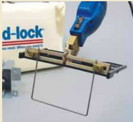
5. The blade holders can accept a wide variety of blades and attachments. The Q-SLED6 is shown.
