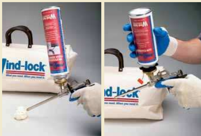
3. Shake can for 1 minute and purge air from gun.
