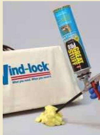
**3.** Shake can for 1 minute and immediately purge the air from gun.
