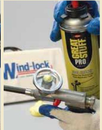
**4.** After removing the can from gun, clean the gun adapter with the Dow® Cleaner.
