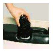
Step 9. If the tank continues to run, remove the FVC and check that the lower piston is in the proper position and check the large o-ring to ensure that it is properly seated. When the vessel is filled and the water stops running, it is an indication that the vessel is filled and ready to continue normal use.
