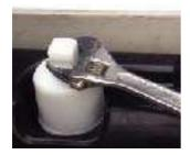
Step 6. Using the tool provided engage the interlocking teeth and rotate the FVC counter clockwise <sup>1</sup>/<sub>4</sub> turn. Then lift the FVC up removing it from the vessel.
