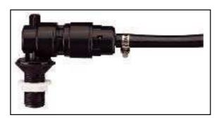
Check lower inlet supply assembly to see if the pressure relief valve is leaking or allowing water to flow into the tank. If water is leaking from the pressure regulator and relief valve of the lower inlet supply assembly, the lower inlet supply assembly must be replaced (EcoFlush Part number B8100-01, covered by factory warranty).
