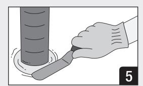
Tool sealant to be flush with substrate.
