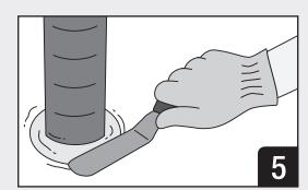
Tool sealant to be flush with substrate.
