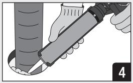
Apply sealant to required depth in annular space per system specifications. Completely fill annular space with sealant.
