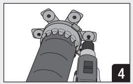
Fix collar to assembly using suitable steel fixings.
