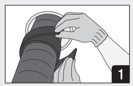
Measure and cut 3M<sup>™</sup> Fire Barrier Wrap Strips FS-195+ or 3M<sup>™</sup> Fire Barrier Wrap Ultra GS to appropriate length for pipe size and layers required as per system specifications.
