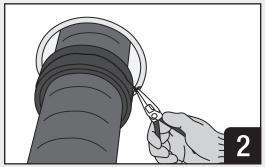
Wrap 3M<sup>™</sup> Fire Barrier Wrap Strips FS-195+ or 3M<sup>™</sup> Fire Barrier Wrap Ultra GS around pipe and position according to system requirements. Secure with steel wire, aluminum foil tape, or equivalent.
