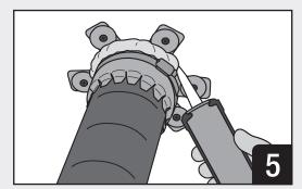
Seal the system with 3M™ Fire Barrier Sealant applied to appropriate interfaces as per system specifications.
