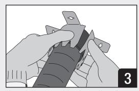
When applicable, secure restricting collar around layers of wrap strip as per system specifications.
