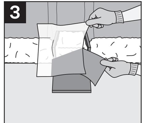
3 Remove second piece of liner, pull tape up around anchor and mullion.
