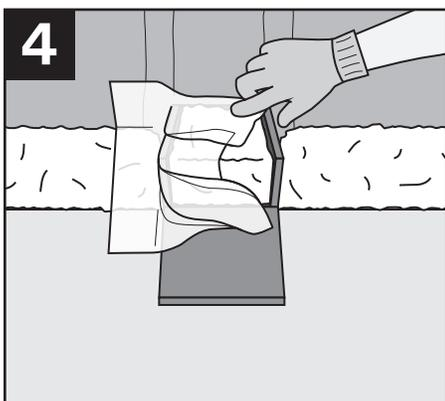
4 Make sure tape has tight seal to curtain wall substrate, following contours of spandrel and framing. The tape will develop wrinkles and leave gaps over the anchor which will be covered by another layer of tape in steps 6–11.
