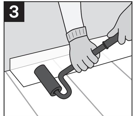
3 Press down firmly with hand or j-roller to adhere tape to surface.
