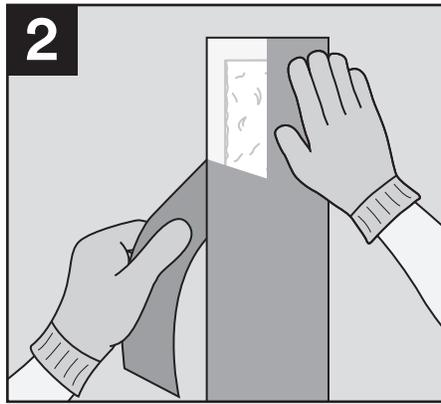
2 Peel back one corner of the liner to expose tape and adhere tape over joint.
