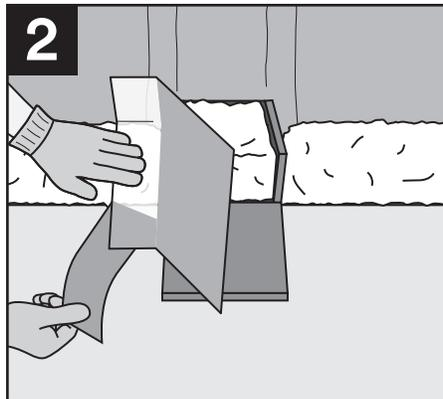
2 Cut a square piece of tape that is at least 2 inches longer than the width of the joint. Fold tape over along the slit liner. Remove skinny liner and press tape into place.
