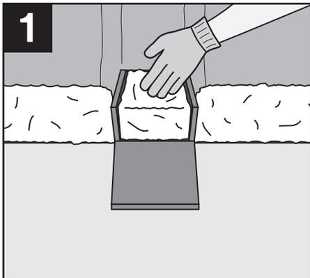
1 Pack mineral wool in between and around areas of anchor that are above the joint.
