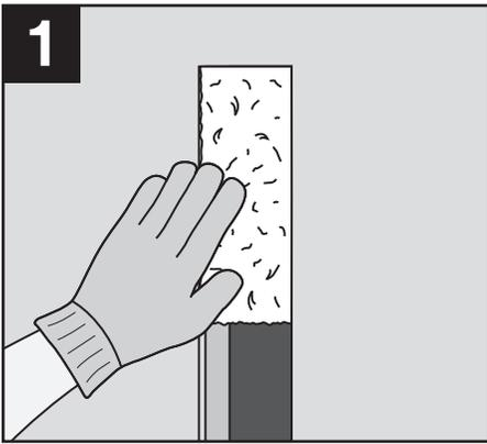
1 Install mineral wool into the straight wall to wall gap.
