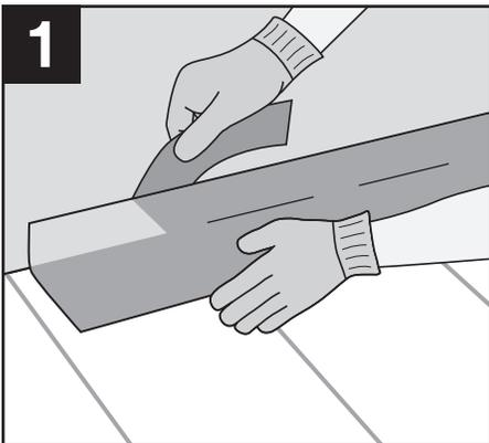
1 Peel back one corner of the liner to expose tape and adhere tape over joint.
