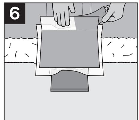
6 Cut a piece of tape that is 2 inches longer than the width of the mullion or anchor (whichever is greater). Peel off skinny piece of liner and press to the vertical section of the mullion or wall above the anchor.
