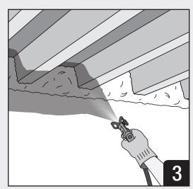
Apply a 3mm thick wet coating of spray to mineral wool, adjacent substrates, and penetrant (if applicable) maintaining all required overlaps per system specifications. Product can also be installed with a brush or roller.
