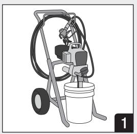
Remove lid from pail and insert pick-up tube from appropriate airless sprayer into 3M™ FireDam™ Spray 200. Prime the pump and set to appropriate pressure for the spray application.\*
