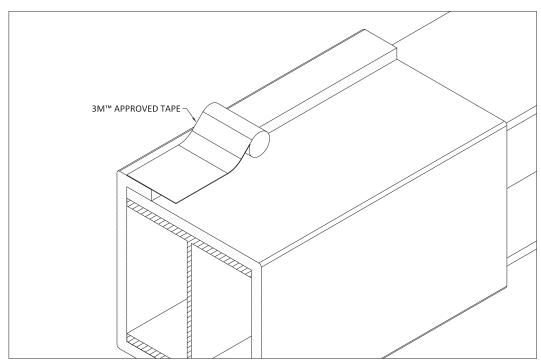
4 - For the next section of wrap, repeat steps 1 through 3. The next section of Emat should be tightly abutted to the first section eliminating all gaps when possible. If a gap of more than 1/8 inch (3 mm) remains in the perimeter joint between sections of EMat, the gap is to be filled to the full depth of the Emat with an approved 3M sealant (Figure 5).
