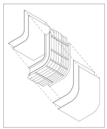
**Figure 5A:** Cut two  $3M^{\text{TM}}$  Interam<sup>TM</sup> Systems E-Mat inner and outer pieces (as shown) to the same width as the cable tray. Secure mat pieces using  $3M^{\text{TM}}$  898 Filament Tape.
