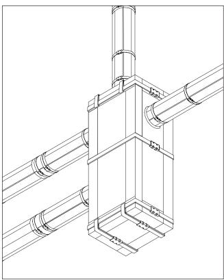
**Figure 4E:** Install steel banding around the box every 12 inches (30 cm) maximum and within 2 inches (5 cm) of each box edge and seam. It may be necessary to attach some banding to other bands, similar to the method shown on the bottom of the box assembly.
