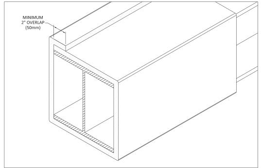
3 - Tape the overlap seam (longitudinal overlap) with approved 3M tape. Center of the tape to be approximately centered over the seam. Smooth the tape with a hard roller or straight edge applying enough pressure to ensure adequate adhesion of the tape to the EMat and to remove any air gaps (Figure 4).
