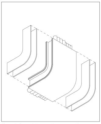
**Figure 5B:** Cut two E-Mat pieces for each side to fit over the cable tray sides and to cover edges of inner and outer E-Mat pieces already installed. Secure mat using 3M<sup>™</sup> 898 Filament Tape.
