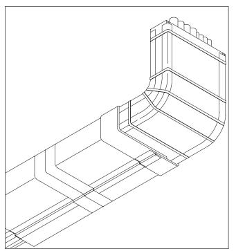
Figure 7G: At the interface between the end of the elbow section and straight section, install a 4 inch (10 cm) wide E-Mat collar centered over the seam with a 2 inch (5 cm) overlap. Secure the mat collar using 3M<sup>™</sup> 425 Sealing Tape.
