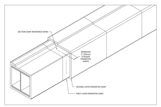
7 - Stagger all subsequent perimeter joints 2 inches from the previous layers' joint. Subsequent layers should be positioned down the longitudinal run so that no two joints align. Repeat steps 1 through 7 for all subsequent layers as per listing/design (Figure 8)
