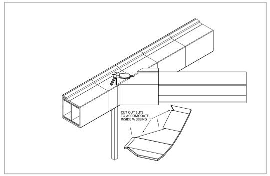
4 - Repeat steps 1 through 3 for all subsequent layers as per listing/design. Once the last layer of Emat is in place, secure the Emat with ½ inch (13mm) wide, 0.020 inch (0.508mm) thick stainless steel banding to be applied over the outside of the wrap.
