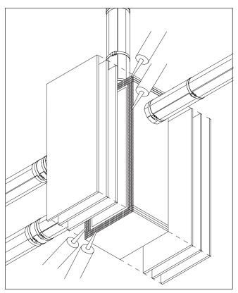
**Figure 4C:** Cut front and back mat pieces large enough to cover front and back of box and the edges of installed mat pieces. Apply 3M<sup>™</sup> Fire Barrier Sealant CP 25WB+ to exposed front and back mat edges and then apply front and back mat pieces. Secure mat using 3M<sup>™</sup> 898 Filament Tape.
