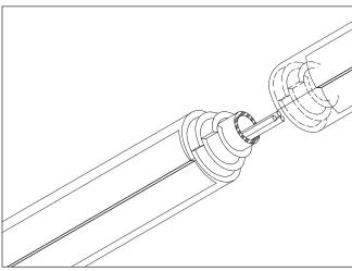
Figure 1D: Install additional layers each offset 2 inches (5 cm) so there are no in-line seams from one layer to another.
