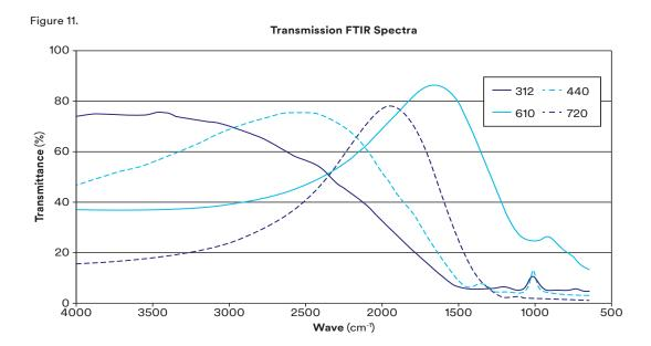
**For Nextel 312:** Between 4000-3250 cm<sup>-1</sup> the transmission loss is small and essentially due to reflection. Weak absorption shows between 3250 and 1500 cm<sup>-1</sup>. Beyond 1500 cm<sup>-1</sup> absorption becomes complete.
