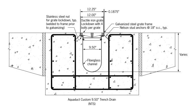
**NOTE:** Concrete and reinforcing steel requirements to be determined by a qualified structural engineer.
