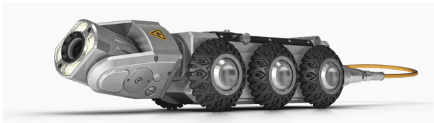
Example of a small-diameter crawler for tight spaces
