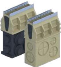
Two-part in-line catch basin with either a plastic base with 4", 6" and 8" drill-outs for pipe connection or a polymer concrete base. Supplied with plastic trash bucket. Options include an in-line or side foul air trap. Available with either galvanized or stainless steel edge rail.
