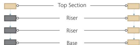
**Base** - Plastic or polymer concrete base available. Plastic bases have a range of SCH 40 4", 6" and 8" cut-outs for easy pipe connection. Cut-outs on end and side allow connection of ACO foul air trap. Polymer concrete bases have drill-outs cast on sides for pipe connections.
