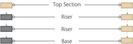
**Base** - Plastic or polymer concrete base available. Plastic bases have a wide range of SCH 40 4", 6" and 8" cut-outs for easy pipe connection. Cut outs on end and side allow connection of ACO foul air trap. Polymer concrete bases have drill-outs cast on sides for pipe connections.
