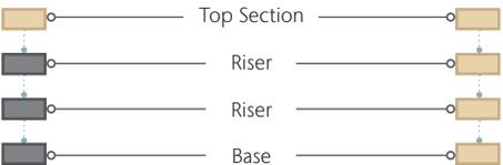
**Base** - Plastic or polymer concrete bases available. Plastic bases have a wide range of SCH 40 4", 6" and 8" cut-outs for easy pipe connection. Cut-outs on end and side allow connection of ACO foul air trap. Polymer concrete bases have drill-outs cast on the sides for pipe connections.
