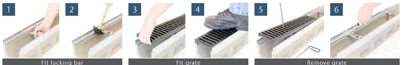
1. Locate locking bar in channel wall recesses by rotating clockwise.
