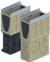
Two-part in-line catch basin with either a plastic base with 4", 6" and 8" drill-outs for pipe connection or a polymer concrete base. Supplied with plastic trash bucket. Options include an in-line or side foul air trap. Available with either galvanized or stainless steel edge rail.
