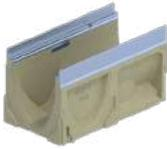
Constant depth channels in 4 depths supplement meter channels. Side knockout and profiling enable side junction to be created. Bottom knockouts on all half meter channels. Available with either galvanized or stainless steel edge rail.
