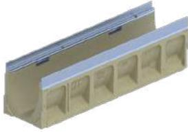
0.5% sloped channels in meter lengths and 40 depths which connect to create 40 meter (131'-2") continuously sloping run. Available with either galvanized or stainless steel edge rail.
