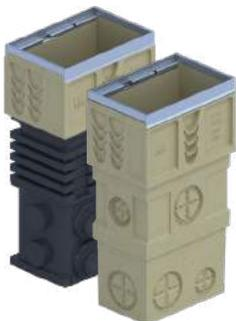
Two-part catch basin; bases have either a plastic base with 4", 6" and 8" drill-outs for pipe connection or a polymer concrete base. Supplied with plastic trash bucket. Optional riser available for increased depth. Available with either galvanized or stainless steel edge rail.
