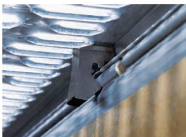
Factory-fitted locking device removes need for bolts and bars and improves channel hydraulic capacity. The DrainLok mechanism clips into channel edge rail for rapid installation. DrainLok grates are fit with an anti-shunt mechanism that restricts unwanted grate movement when installed, improving durability and longevity of the system.
