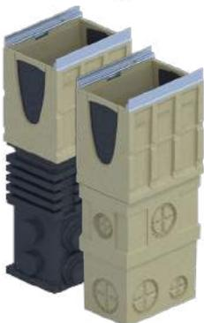
Two-part in-line catch basin with either a plastic base with 4", 6" and 8" drill-outs for pipe connection or a polymer concrete base. Supplied with plastic trash bucket. Available with either galvanized or stainless steel edge rail.
