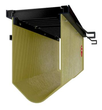
FG200 is an 8" wide fiberglass system with choice of steel slotted Class C (25 ton) or ductile iron Class E (60 ton) grates. Grates are bolted into the steel frame with 2 bolts per 18" section.
