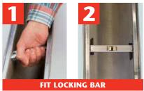
Locate locking bar in recesses, rotate and use hammer to tap securely into place. Serrated ends grip in recess.
