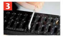
To close, place hook part of tool into 'V' and push towards rail.
