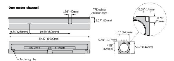
Slot channel trench drain system with cellular rubber
