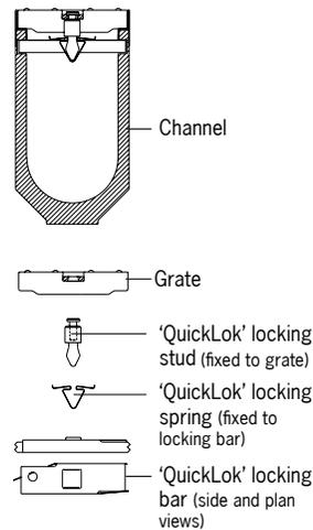
ACO 'QuickLok' is a patented boltless locking system, grates are removed and replaced with the minimum time and effort for ease of maintenance. The unique design provides a positive 'snap down' fit into the locking bar. A stud is fixed to the grate which 'locks' into the spring clip in the locking bar.
