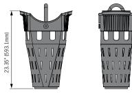
Note: Openings in trash bucket are 74.4"2 (48,028mm<sup>2</sup>)
