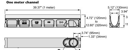
3.94" (100mm) 3.94" (100mm) Half meter channel 11.81" (300mm) 19.69" (0.5 meter)
