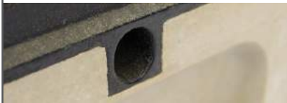
Concrete Anchor Boss A drill-through hole in the ductile iron rail enables a concrete anchor (4 per meter) to be attached for extra embedment into concrete haunch.
