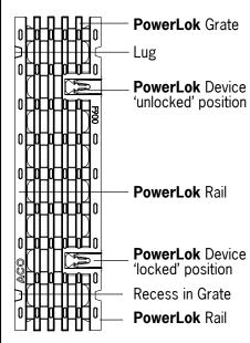
ACO PowerLok is a patented boltless locking system. Grates are removed and replaced with minimum time and effort for ease of maintenance.
