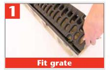
Position grate onto channel, align holes in grate with matching holes in edge rail. Using wrench or socket set to tighten. If using a torque wrench, do not set to more than 15 ft. lbs.
