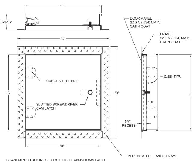
STANDARD FEATURES: SLOTTED SCREWDRIVER CAM LATCH 5/8" RECESSED DOOR PANEL SATIN COAT STEEL, MILL FINISH
