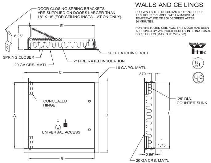
UNIVERSAL SELF LATCHING BOLT- OPERATED BY KNURLED KNOB / FLUSH KEY, WITH INSIDE TURN RELEASE. CARBON STEEL, PRIME COAT BAKED ENAMEL FINISH STANDARD FEATURES:
