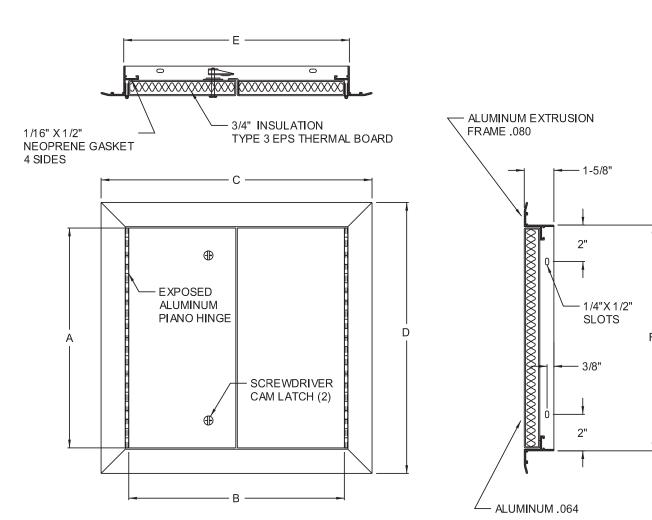
STANDARD FEATURES: SCREWDRIVER OPERATED CAM LATCH, ALUMINUM DOOR AND FRAME, MILL FINISH 0PTIONS: 1/16" X 1/2" NEOPRENE GASKET 4 SIDES OPTIONS: MATERIAL **FINISH** LOCK TYPE
