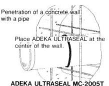
At the center of the wall, apply Adeka Ultraseal ® P-201 uniformly without any gaps. To obtain a bead which is 20mm (5/6 inch) wide and 5mm (1/4 inch) thick, cut the tube at the first line.
