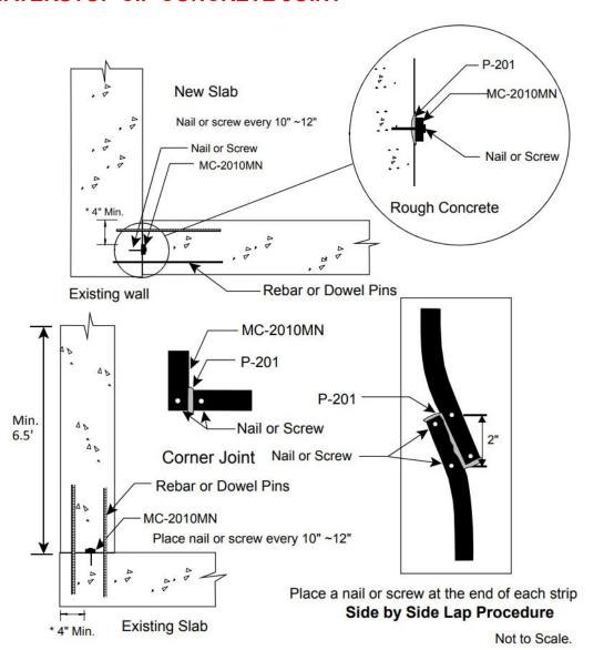
IMPORTANT: The recommended minimum concrete coverage is 4". This is a safety factor for unknown concrete quality and compacting techniques. Call your local ADEKA ULTRASEAL ® Representative or (800) 999-3959 for exact coverage details.
