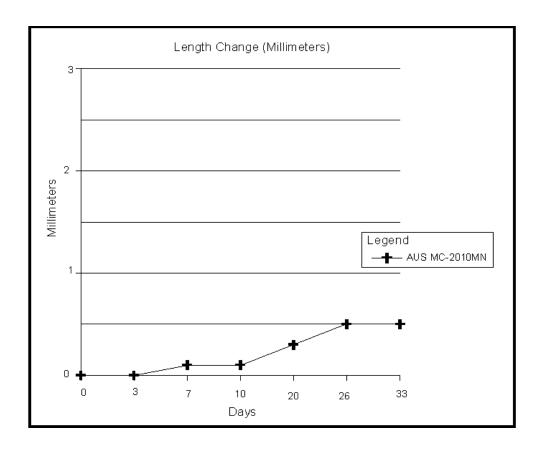
As shown, length expansion is limited to an insignificant amount. The addition of the stainless steel net to the MC-2010MN controls the expansion direction and pressure. Expansion is directed to the vertical plane. This is where waterstopping function is most critical. If unintentional hydration occurs before the waterstop is covered, winding or warping of the product is prevented by the wire net. Expansion is focused in the width direction by the wire mesh.
