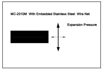
Some products that have a high amount of expansion occurring before concrete is cured can leave a gap or void between the concrete and the waterstop. This will create a path for water penetration. Also higher expansion requires more concrete coverage to prevent concrete "blow-outs".
