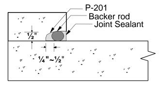
No. 1: For P-201 repair - cut a notch 1/2" X 2" deep
