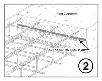
2. After first concrete is placed, remove any concrete that protrudes past the expanded metal form along the line of the first P-201 application.
