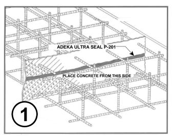
1. Apply a uniform  $\frac{1}{4}$ " X  $\frac{1}{2}$ " bead of Adeka P-201 to the metal form on the first concrete placement side.
