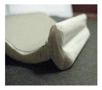
After applying the P-201, spread and even the P-201 by pushing the tool through the interlock. Use a steady even forward motion.
