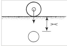
cover of at least 12" (0.3 m) for 4" - 48" (100-1200 mm) diameters and minimum cover of at least 24" (0.6 m) for 60" (1500 mm) diameters.
