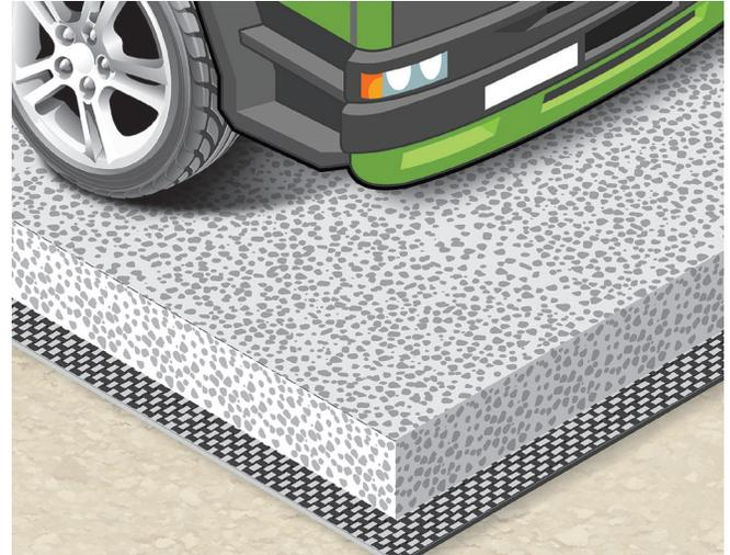
**ADS woven geotextiles can reduce aggregate thickness in unpaved roadways. The geotextile stabilizes roads by spreading loads over a wider foundation, reduces rutting and prevents contamination by the subgrade soil.**
