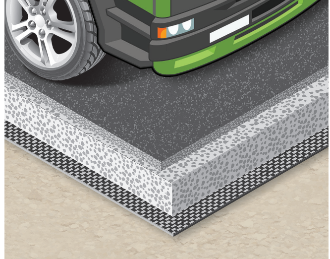
Paved roads and parking lots have a longer expected life with the use of an ADS woven geotextile, which will permanently separate the subgrade from the aggregate.
