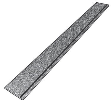
C. Once separated, the Shingle Starter strips should be aligned next another, with the sealant toward the eave.
