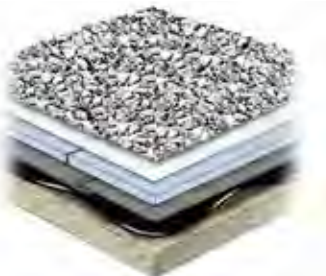
Stone Ballasted Protected Membrane Roof
