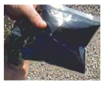
Combine/mix the two components together, inside the plastic bag, by kneading the bag for a MINIMUM OF FIVE (5) MINUTES.
