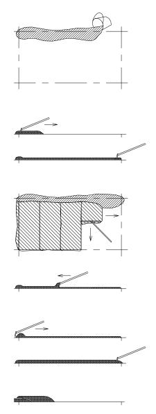
This technique typically requires a minimum of three passes over the same area to properly work the membrane to assure that it be installed to the specified thickness. Even in cold weather, there should be sufficient time to make the three passes as outlined in the above technique.
