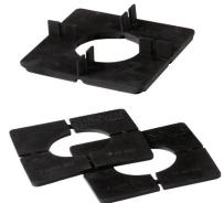
The flexible pedestals can be used singularly or in combination with the shims to accommodate elevations from 3/8 inch to 2 inches. Shims can be used with the support pedestals in whole, or cut into halves or quarters for minor leveling and elevation adjustments. The flexible pedestals cannot be stacked together.
