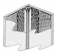
Refer to ASTM C1063 for support spacing, lath selection, fastener selection and further information regarding the proper installation of metal lath.
