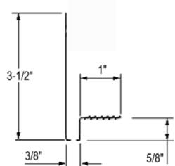
FIRE TESTING: The assembly including C-I Weep Trac™ meets NFPA 285-Standard Fire Test Method for Evaluation of Fire Propagation Characteristics of Exterior Non-Load-Bearing Wall Assemblies Containing Combustible Components.
