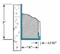
**AMICO EIFS Starter Track/Casing** (Without Drip Edge) and with Drainage Holes can be installed at the bottom of the wall as a starter track, but is usually installed around the perimeter of the wall as a casing to protect the edge of the foam board and finish from damage and the elements. This product does not have a drip edge. Ridges and perforations on the face of this bead aid in finish adhesion. Excellent adhesion of EIFS finishes and paint can be expected with all AMICO vinyl EIFS beads.
