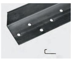
J-Metal Bead is used with one-coat stucco systems or thin veneer stone. Optional holes in ground are spaced at 6" centers.
