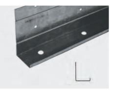
**Foundation Weep Screed (FHA #7)** is required at the base of walls as part of a drainage system for exterior stucco or veneer stone applications. The 3½" nailing flange serves as flashing when Grade D building paper or Tilath™ Starter Strip is installed over the flange. Holes are punched into the nailing flange for easy attachment to the wall. Holes are also placed on top of the "V" portion of the flange to provide keying of the stucco mud when wet.
